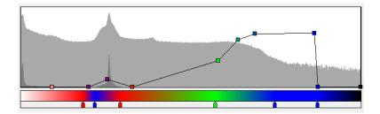
Figure 2.4: Transfer function widget; density values increasing from left to right, the different colors at the bottom visualize the colors to which the density values will be mapped. The line above it shows the level of transparencies; in the background a histogram of all voxel values is shown.
