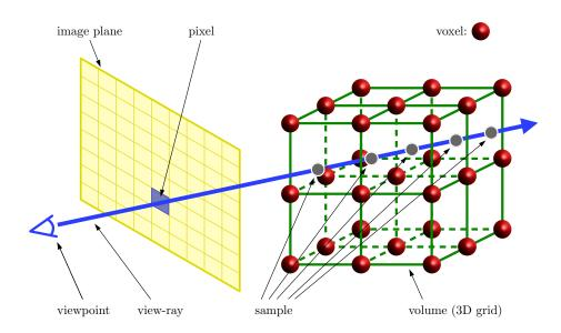
Figure 2.1: Illustration of ray casting
