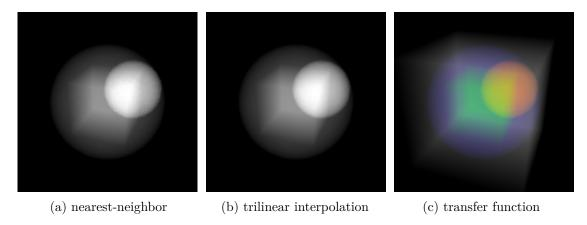
Figure 7.1: Encrypted rendering results; Volume size:  $100 \times 100 \times 100$  voxels; Image size:  $150 \times 150$  pixels (the shown images are scaled by LATEX)
